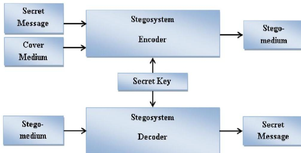
**Figure (2.1): Steganography System Architecture**
